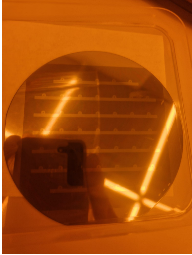
(a) The image is showing the wafer after development. The black area around the antenna is the hardened photoresist.
