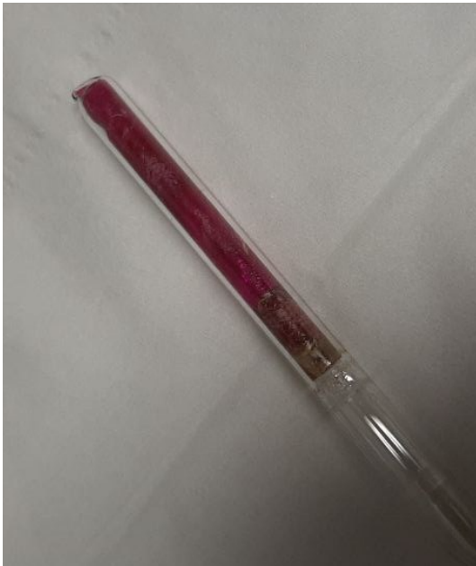
(a) PC:PTP crystal grown at 270 °C. The inhomogeneity can be observed due to insufficient mixing of the substances before placing them in the furnace.
