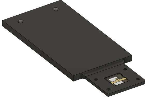
Figure 3.5: CAD design of the antenna in the sample holder.
