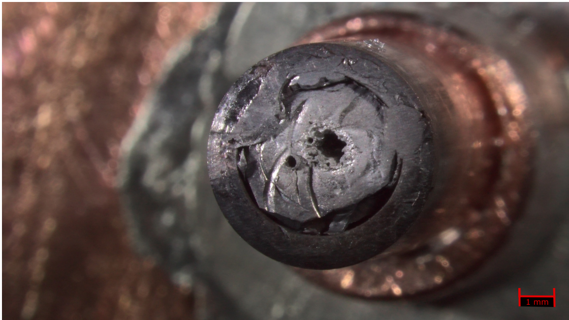
Figure 4.10: Ytterbium target after all the measurements were taken, with roughly three thousand shots.
